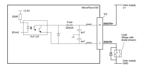
Figure 30 - DOUT0 output circuit
